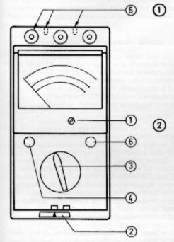
With the current cut off check the zero position adjustment of the pointer. After cleaning the scale window the eleccharge trostatic should be neutralized by breathing on the glass or touching it or wiping it with a damp cloth.
